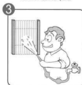
Clean the mesh with water sparying
